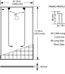
(A) Cable Length: 48.2 in +/-0.4 in [1225 mm +/-10 mm] (B) Long Side: 1.3 in [32 mm] Short Side: 0.9 in [24 mm]
